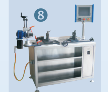
Z-25104: EPS-R Electric racks Cremagliere elettriche (es. VW Golf V, Toyota, Nissan)
